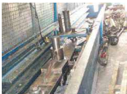
» Proof Load Test on steel parts
