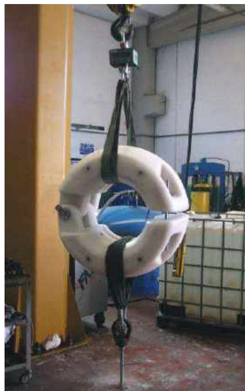
» Tension Test on float assembly
