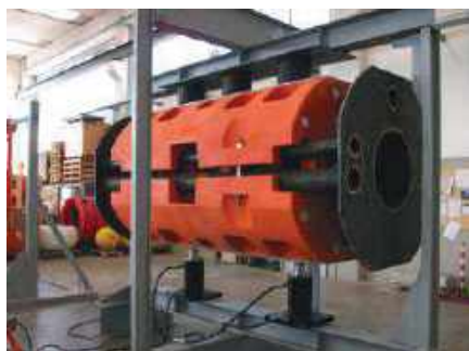
» Structural Pressure Test on the buoy body
