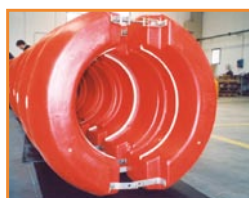
Historical hinged type Resinex floats with reduced width collar
