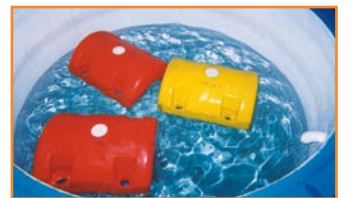
Floats after pressure test still in autoclave
