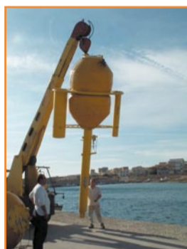
View of lateral chambers for sensors
