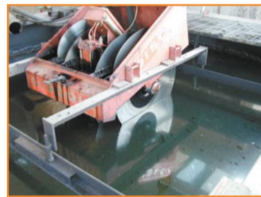
The skimmer during test
