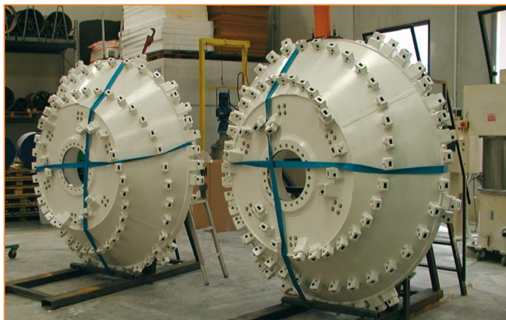
The excavation cutters during filling with Synt 3000
