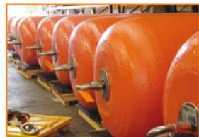
The complete package was supplied by Resinex in the Spring of 2004 even if the feasibility and resistance studies required many months of work by the Resinex Technical Office before consignment. It needs to be noted that all the metallic parts used are in stainless steel AISI 316, which together with all the standard Resinex fenders (high density polyethylene and the high abrasion resistance elastomer polyurethane) guarantee a limited level of maintenance and a high level of safety.
