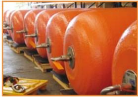
The complete package was supplied by Resinex in the Spring of 2004 even if the feasibility and resistance studies required many months of work by the Resinex Technical Office before consignment. It needs to be noted that all the metallic parts used are in stainless steel AISI 316, which together with all the standard Resinex fenders (high density polyethylene and the high abrasion resistance elastomer polyurethane) guarantee a limited level of maintenance and a high level of safety.
