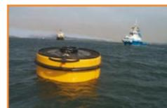
a convenient and strong mooring point. Resinex has supplied directly to the Olbia Port Authority, through Stemasub, four Big Pem 30 mooring buoys destined to be positioned at the Industrial Port and at the Isola Bianca of Olbia for the mooring of big ships. The buoys, which have been tested for a mooring of 75 tons, have a diameter of 3 meters and a buoyancy of 7700 kg.
