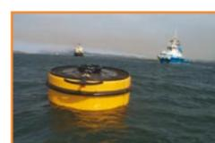
a convenient and strong mooring point. Resinex has supplied directly to the Olbia Port Authority, through Stemasub, four Big Pem 30 mooring buoys destined to be positioned at the Industrial Port and at the Isola Bianca of Olbia for the mooring of big ships. The buoys, which have been tested for a mooring of 75 tons, have a diameter of 3 meters and a buoyancy of 7700 kg.
