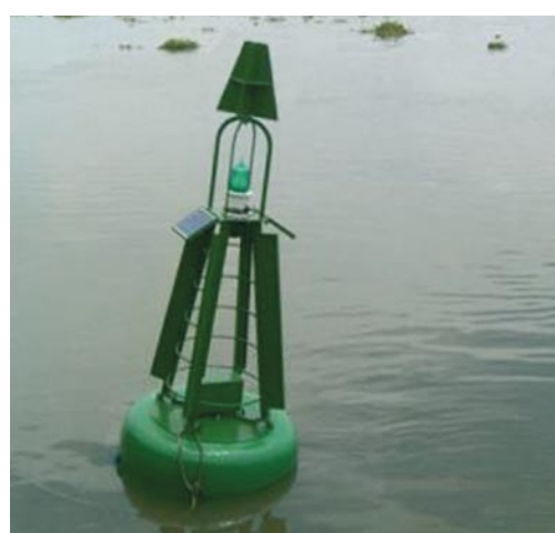
Stability: under traction tests the buoy tilts only a few degrees.
