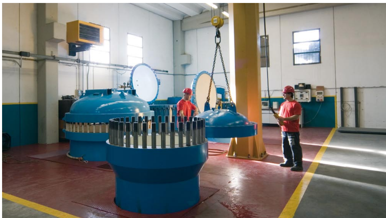
In these 5 big autoclaves we test the deep water floats until 400 Bars.
