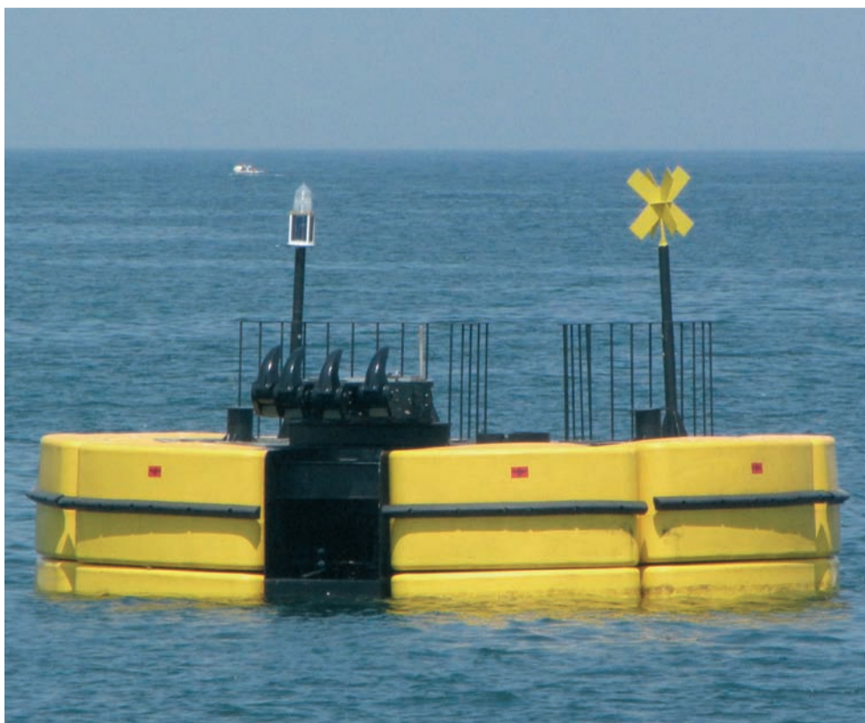
The buoys have a quadruple hook for mooring.
