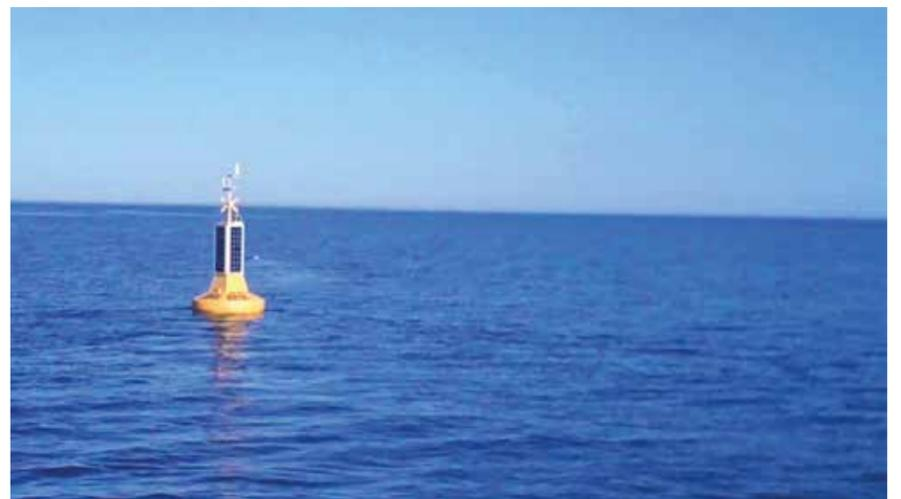
be adopted in the Bosphorus, in Antalya Port and in Tasucu Port. The above mentioned buoys, besides giving a constant meteo monitoring, are able to make a considerable variety of surveys: from the water salinity, to the marine current measurements, passing through the wave measurement and the tsunami prevention.
