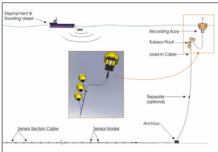
Above: working scheme of the RXT sensor system for the sea bed detections.
