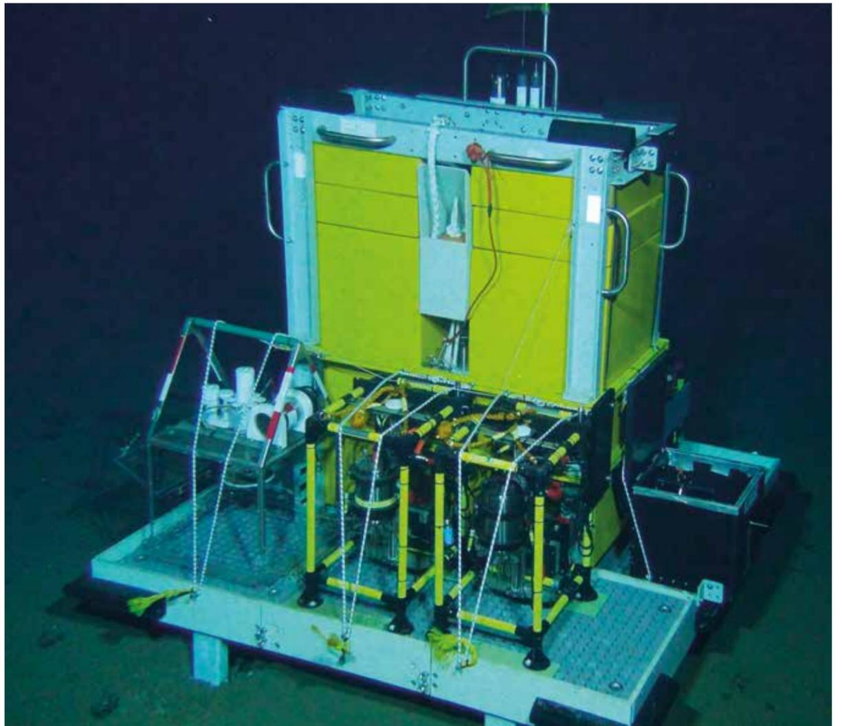
In the middle of the elevator a box with a Resinex floatation line is visible, which can be released by the ROV pulling the orange line to facilitate the recovery
