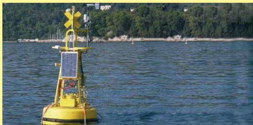
The National Institute of Oceanography and Experimental Geophysics (OGS) of Trieste has installed an instrument monitoring buoy in the Otranto canal as part of a European project. This is a floating system connected to a depth of 1200 metres and fitted instruments and sensors in order to carry out profiles of the wind and water. For this project a Resinex model PEM 18 buoy was used with a float of 1.8 metre diameter with a signalling lantern. The power is guaranteed by solar panels.
