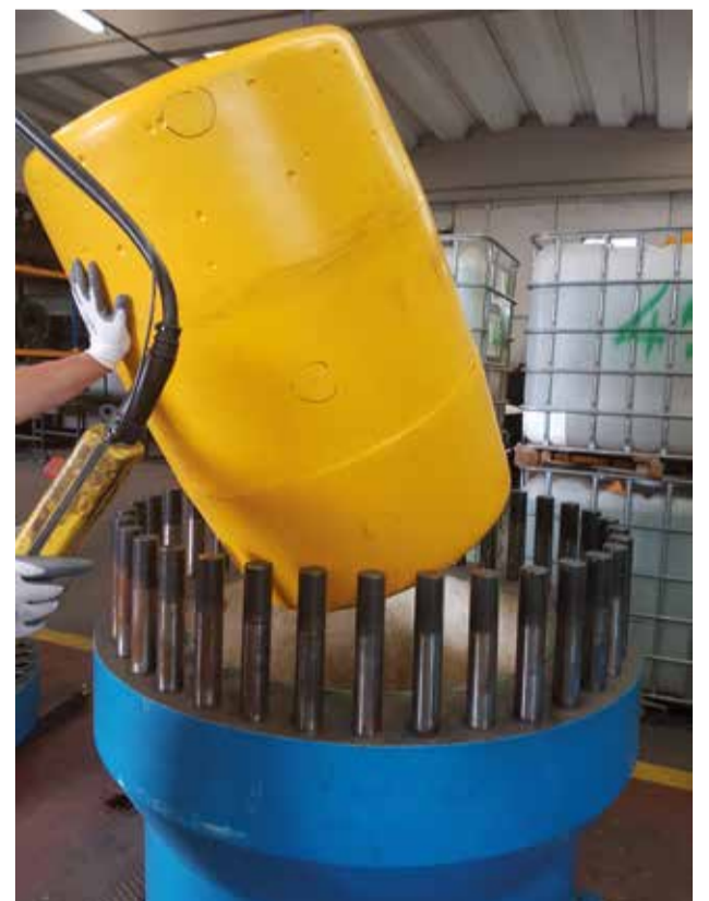
Hydrostatic pressure test
