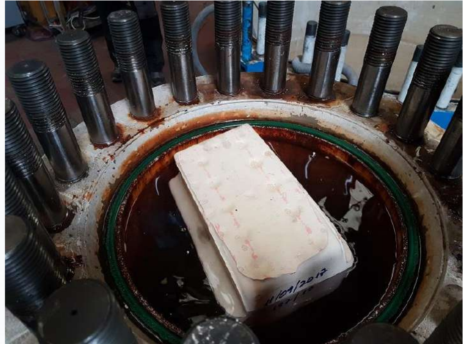
Hydrostatic pressure test – till 950 bar
