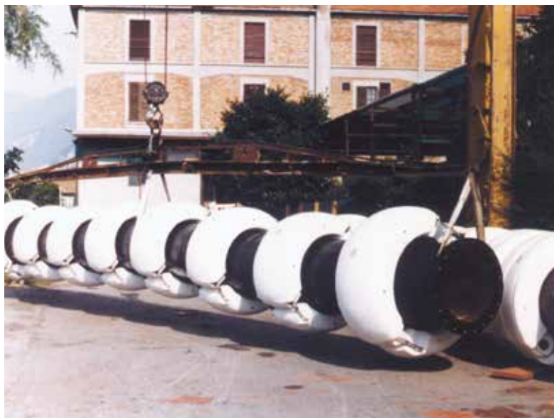
Assembling test of a complete float set for rubber hose in house.
