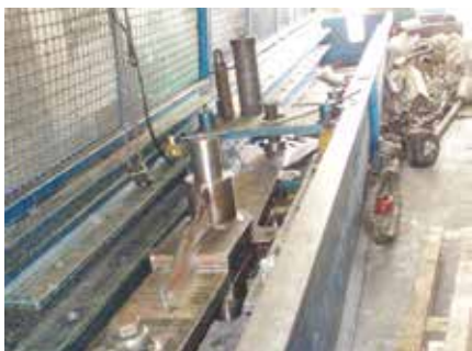
» Proof Load Test on steel parts
