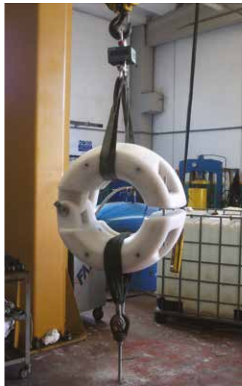
» Tension Test on float assembly
