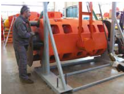
» Impact Test on the buoy body
