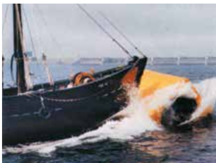
» Crash Test on buoyancy elements
