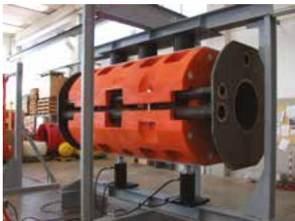
» Structural Pressure Test on the buoy body
