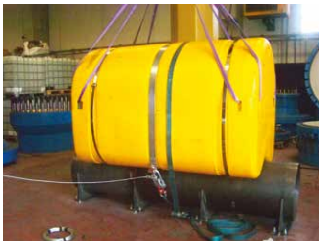
» Fastening Removal Test on Pipe Floats
