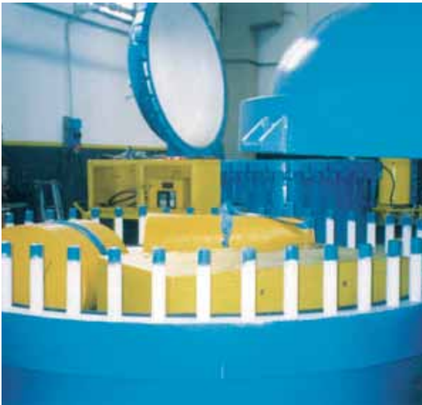
Pressure tanks for high depth tests
