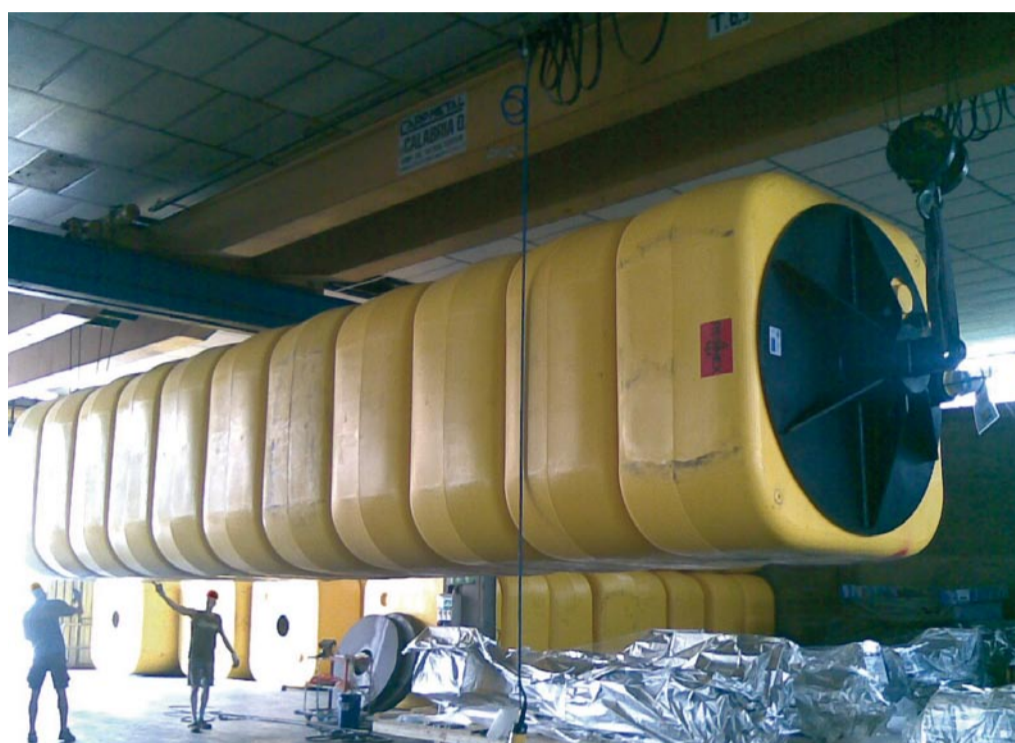
Above: assembling tests and final checks for the modular buoy: it is 12 metres long. Below: a module after the test pressure in the autoclave.
