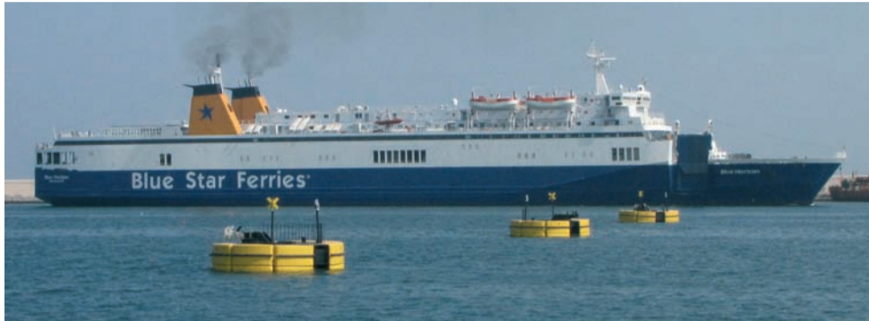
Every buoy has a diameter of 5,8 metres and weighs 16 tonnes.
