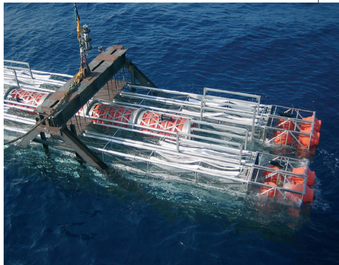
The Nemo module with by Resinex orange buoys 4000 meters water depth rated.
