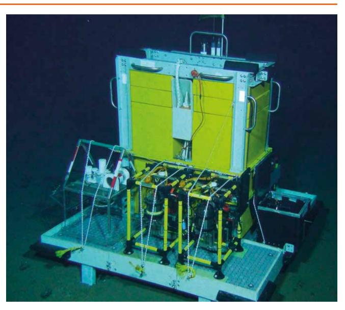
In the middle of the elevator a box with a Resinex flotation line is visible, which can be released by the ROV pulling the orange line to facilitate the recovery
