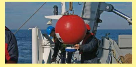
The National Institute of Oceanography and Experimental Geophysics (OGS) of Trieste has installed an instrument monitoring buoy in the Otranto canal as part of a European project. This is a floating system connected to a depth of 1200 metres and fitted instruments and sensors in order to carry out profiles of the wind and water.
