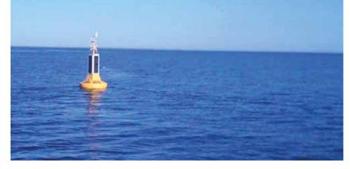
be adopted in the Bosphorus, in Antalya Port and in Tasucu Port. The above mentioned buoys, besides giving a constant meteo monitoring, are able to make a considerable variety of surveys: from the water salinity, to the marine current measurements, passing through the wave measurement and the tsunami prevention.
