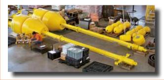
with solar panels autonomous power supply system, with wireless link for data communication, Gps receiver, signalling light and radar reflector Iala compliant. The stability of the Spar configuration allows to get reliable acoustic communication also in case of high sea states. The implemented system allows to increase the safety of the Thai coasts providing an alarm one hour in advance in case of detection of anomalous waves over the normal tide.
