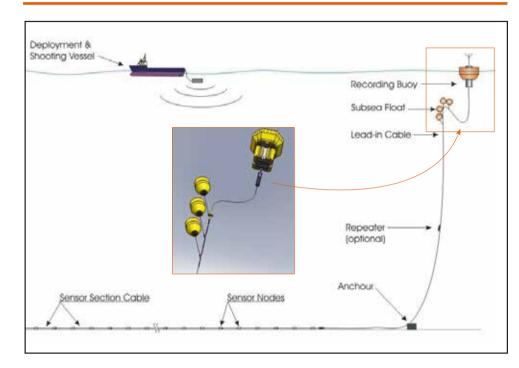
Above: working scheme of the RXT sensor system for the sea bed detections. Right: the installation of the Resinex buoys. Reservoir Exploration Technology (RXT) was a Norwegian company extremely specialized, with branches all over the world.
