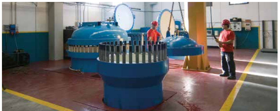
Tanks for hydrostatic pressure, hydrostatic crush and net buoyancy tests
