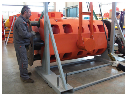
» Impact Test on the buoy body
