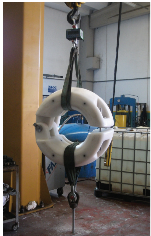
» Tension Test on float assembly
