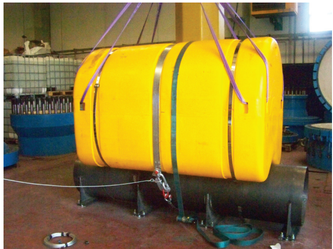
» Fastening Removal Test on Pipe Floats
