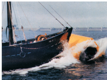
» Crash Test on buoyancy elements
