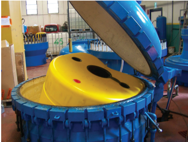
» Hydrostatic Pressure Test in 6 pressure tanks till 850 bars
