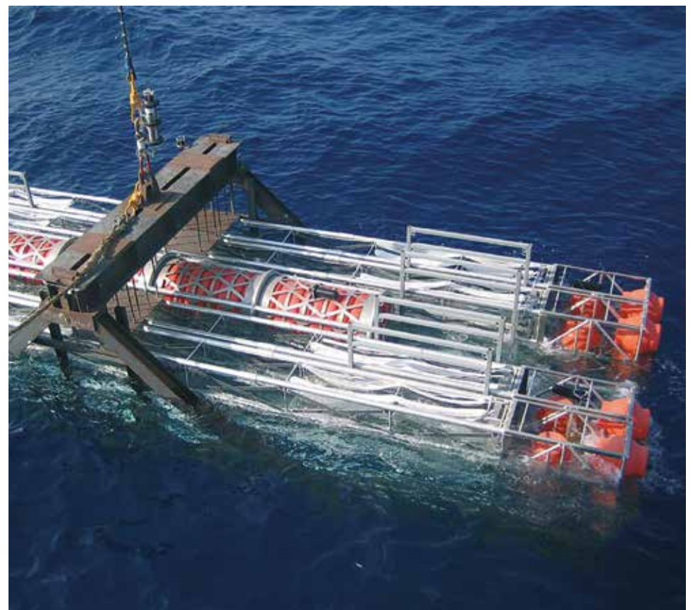
The Nemo module with Resinex orange buoys rated 4000 metre water depth.
