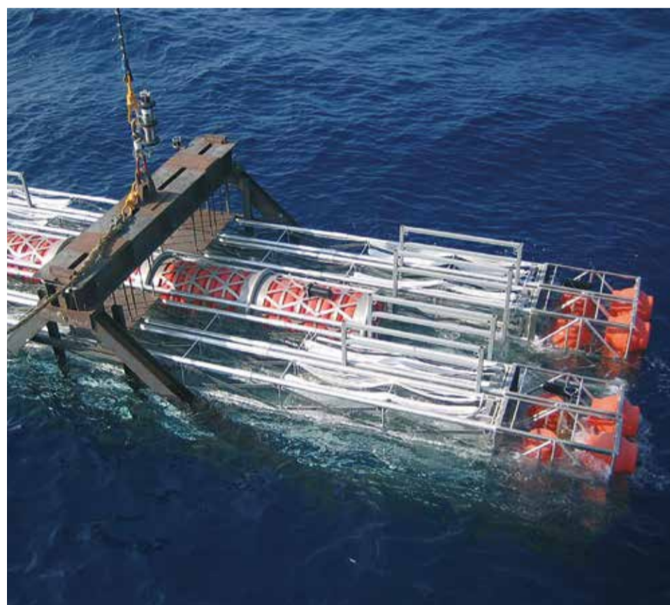
The Nemo module with Resinex orange buoys rated 4000 metre water depth.
